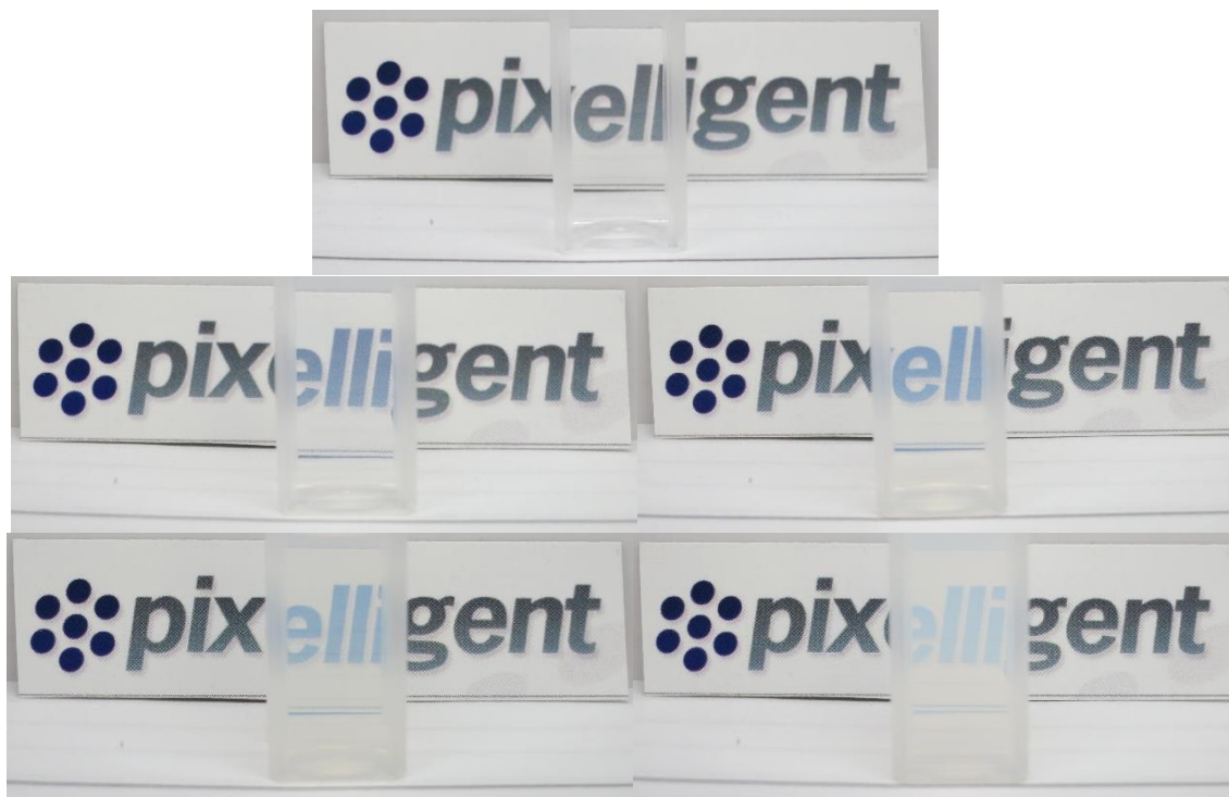
Figure 1. Top picture, PGMEA solvent in a cuvette. Below, examples of PixClear® dispersions with different compatibility levels: clear, slightly hazy to very hazy. All cuvettes have 1 cm path length.
