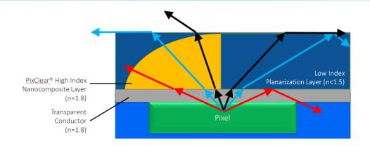
More importantly, the high refractive index layer can match the index of the transparent conducting layer and the light emitting region of the OLED device, minimizing the loss of light due to total internal reflection. Based on a simple optical model we estimate the improvement in light extraction efficiency at 50% to 200%.
