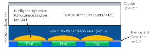
The lens has to have a high refractive index so that the curved surface is capable of forward focusing light when embedded in a low index planarization layer, improving the useful brightness of the display as more light is directed towards the common viewing angles<sup>3, 4</sup>. The performance can be engineered through the detailed lens shape and curvature design as well as by co-optimizing the pixel design.
